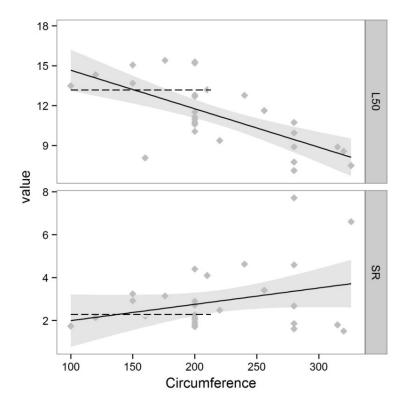
Figure 17. Relationship between selectivity parameters (L50% and SR) and codend circumference for *M. barbatus*. Solid line represents DM codends, dashed line represents average value for SM codends.
