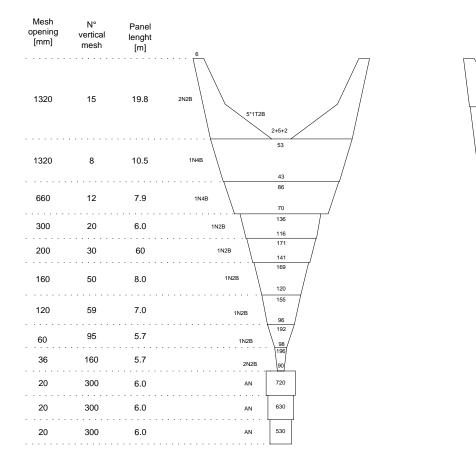
Figure 68. Original design of the single-boat pelagic trawl.
