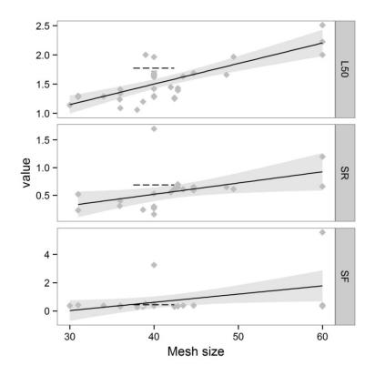
Figure 19. Relationship between selectivity parameters (L50% and SR) and mesh size for *P. longirostris*. Solid line represents DM codends, dashed line represents average value for SM codends.
