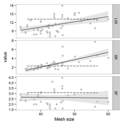
Figure 16. Relationship between selectivity parameters (L50% and SR) and mesh size for *M. barbatus*. Solid line represents DM codends, dashed line represents average value for SM codends.
