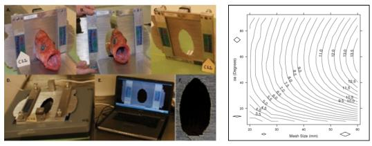
Figure 8. Fish being measured using FISHSELECT morphometer *(left)*; example on Design Guide for diamond meshes for a specific species *(right)*. It shows ISO curves for the size of fish that based on morphology would be able to escape through diamond meshes of different mesh size (*X*-axis) and different opening angle (*Y*-axis).
