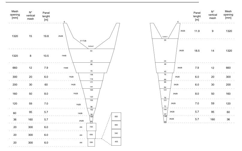
Figure 69. Modified design for the meshing experiment. The four netting sections have been inserted before the last netting piece of the codend.
