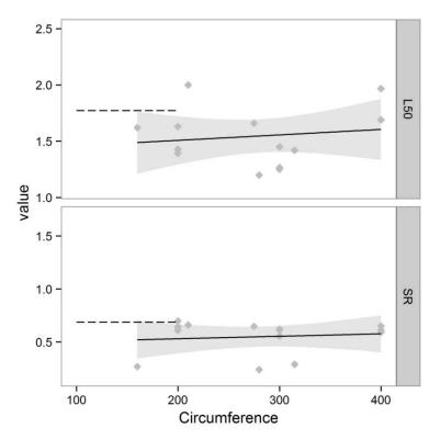
Figure 20. Relationship between selectivity parameters (L50% and SR) and codend circumference for *P. longirostris*. Solid line represents DM codends, dashed line represents average value for SM codends.
