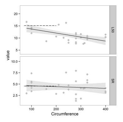
Figure 14. Relationship between selectivity parameters (L50% and SR) and codend circumference for DM codends for *M. merluccius*. Solid line represents DM codends, dashed line represents average value for SM codends.
