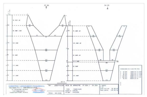
Figure 42. Schematic diagram of the commercial bottom trawl net used on the shallow shelf fishing grounds during the short pilot action developed off Menorca (Balearic Islands, western Mediterranean).
