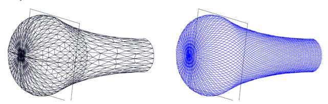
Figure 29. View of the model of codend. The net is split into contiguous triangles in the modelling. On top the triangular element are shown when on the bottom the twines are shown (only 1 on 10 twines is shown). This figure corresponds to  $p_d_ms_30_tt_10_ma_800$  (see deliverable *D 0.2. Geometry of the codends*) and a catch of 5000 kg.
