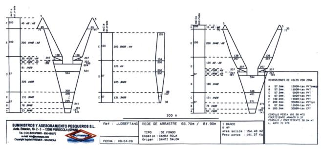
Figure 43. Schematic diagram of the commercial bottom trawl net used on the middle slope fishing grounds during the short pilot action developed off Menorca (Balearic Islands, western Mediterranean), within the framework of DISCATCH project.
